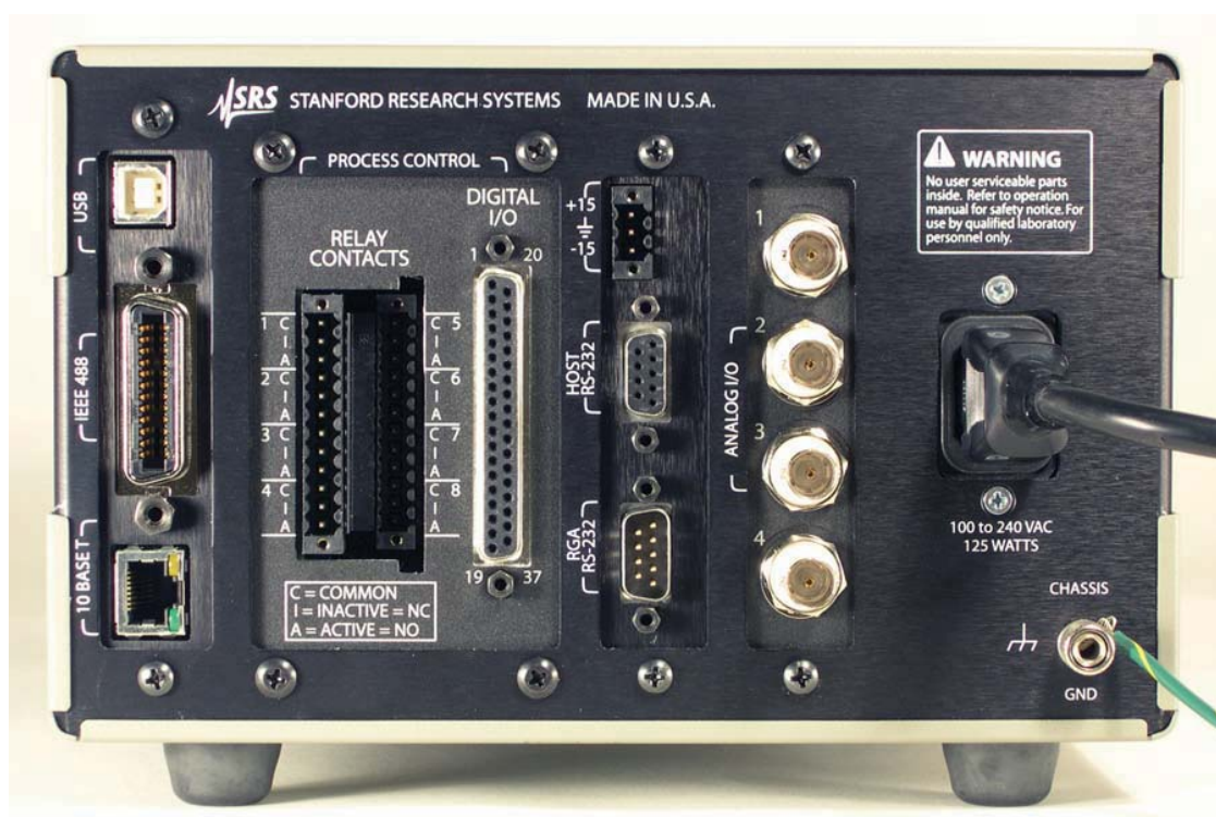
Figure 2. Back panel of the PPM100 controller. Connect the SRS RGA to the RGA RS-232 (DB-9) connector using a standard serial communication cable.
