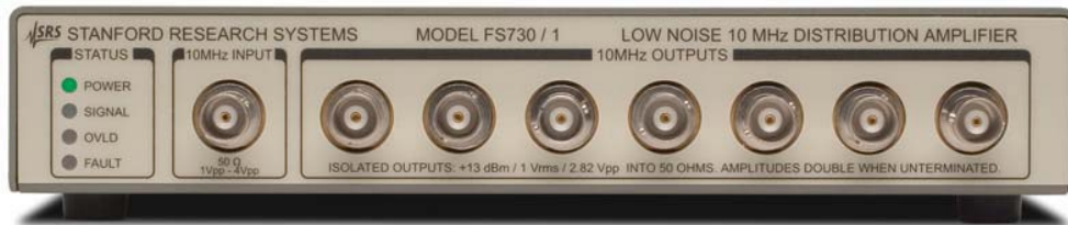
Figure 5. Single 10MHz Distribution amplifier, FS730/1. The FS735 dual distribution amplifier is also available.
