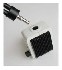
The light guide is inserted into the light guide socket as far as the stop (1). To ensure a tight fit and optimum illumination the groove must click into the retaining slot.
