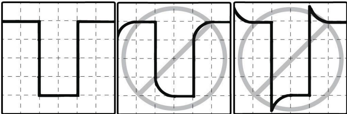
\*The probe can not meet the full specification if under or over compensated or incorrectly adjusted. The better compensated, the flatter the frequency response and higher bandwidth you will obtain.
