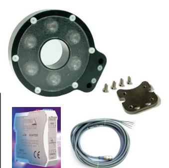
Light includes LDM DIN rail mount constant current driver, 4-meter cable and hardware to mount to Cognex Insight 5100 series camera (driver is available with variable or 0-10VDC intensity control - cable also available in 8, 15 and 30-meter lengths)
