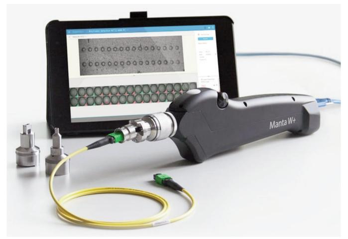
The SUMIX Manta-W+ is a revolutionary portable microscope designed for inspection of all types of single and multi-fibre optical connectors, patch cords and bulkhead, included but not limited to: MT, MPO, LC, FC, SC, CS®, E2000<sup>™</sup>, PRIZM, QSFP, ARINC, MIL Spec termini, ODC12, high-power SMA, Avim, mini-Avim and more.
