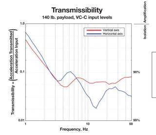
**Caution!** Be careful when comparing our performance to alternative designs. Our data is actual measured performance, not a model. Furthermore, the data is taken with only lowamplitude, micron level vibration as the excitation.
