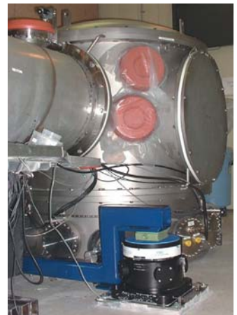
STACIS® supporting the end chambers of a prototype LIGO interferometer at the California Institute of Technology. These are the most precise instruments ever made – capable of measuring distances of less than 10 -18 m.
