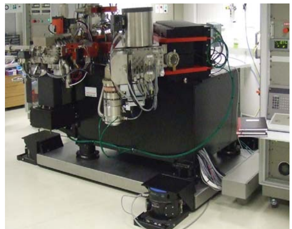
A Cameca NanoSIMS 50L on a TMC 65 Series Floor Platform supported by STACIS ® isolators. This tool is a 5,000-pound secondary ion mass spectrometer with a spatial resolution of 50 nanometers. Photo courtesy of the Planetary and Space Sciences Research Institute (PSSRI) at The Open University, Milton Keynes, U.K.
