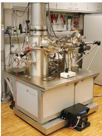
65 Series STACIS ® Floor Platform supporting an Omicron Multiprobe Scanning Tunneling Microscope (STM) with nanometer scale resolution at the Max Planck Institute in Dresden, Germany.
