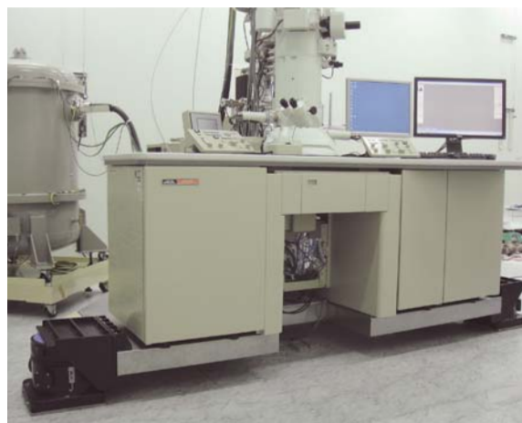
STACIS ® 65 Series Floor Platform supporting a JEOL JEM-2100F Transmission Electron Microscope (TEM).
