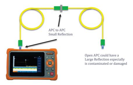
Mated APC connections have very low reflectivity (<65dB typical) An open (not connected) APC could have a higher reflectivity (~45dB)
