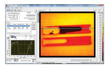
Line Profile: The ROI window graph on the lower left shows the pixel intensity profile along the horizontal green line on top of the image of the upper cuvette. This cuvette holds both water and used motor oil, while the lower one just has oil. SWIR imaging through a 1475 nm bandpass filter causes the water to appear black while the oil is red and airbubbles in yellow in this pseudo-colorized image.
