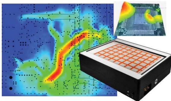
EMC and signal integrity are major concerns in the design of ultra-high speed (>2 GHz) PCBs. EMScanner enables the design engineers to diagnose EMC/EMI problems between 150 kHz and 8 GHz.
