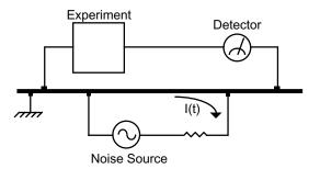
In this illustration, the detector is measuring the signal relative to a ground far from the rest of the experiment. The experiment senses the detector signal as well as the voltage from the noise source's ground return current, which passes through the finite resistance of the ground between the experiment and the detector. The detector and the experiment are grounded at different places which, in this case, are at different potentials.
