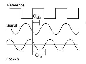
The lock-in amplifies the signal and then multiplies it by the lock-in reference using a phase-sensitive detector or multiplier. The output of the PSD is simply the product of two sine waves.
