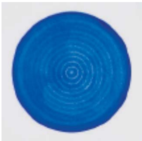
Figure 1. Vibration-induced concentric ring pattern in a 100mm dish containing chick embryo fibroblasts that was stained 1 hour after plating.
