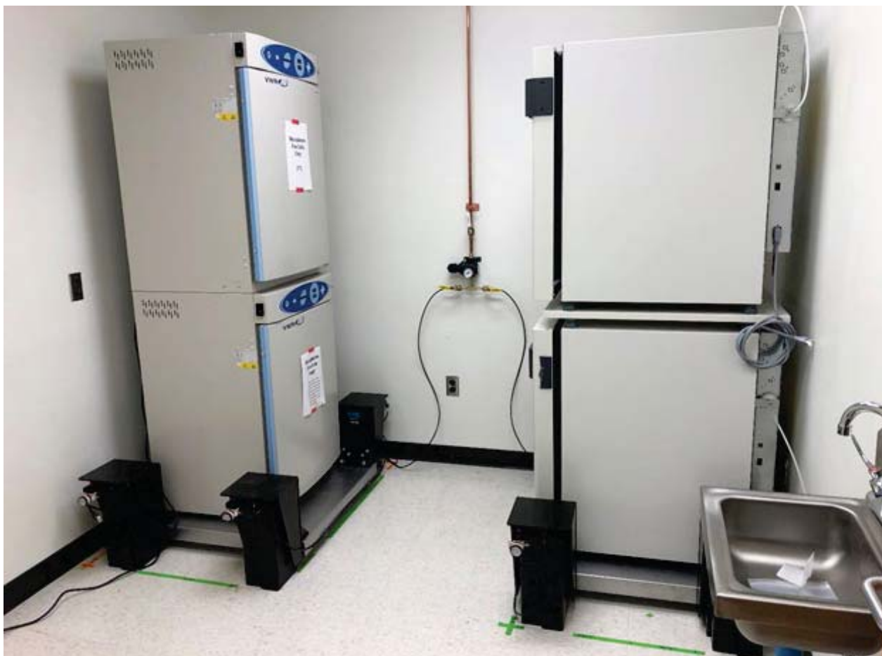
Figure 3 Incubators stacked on TMC MaxDamp vibration isolation platforms
