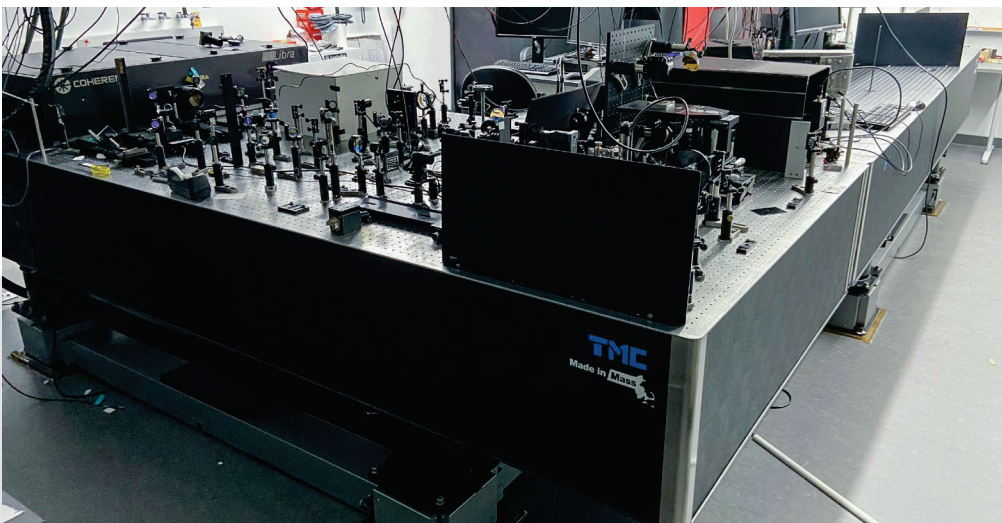
Shown is the LaserTable-Base with the L-shaped design that's used by the Ultrafast THz and Optical Spectroscopy Lab at WPI.
