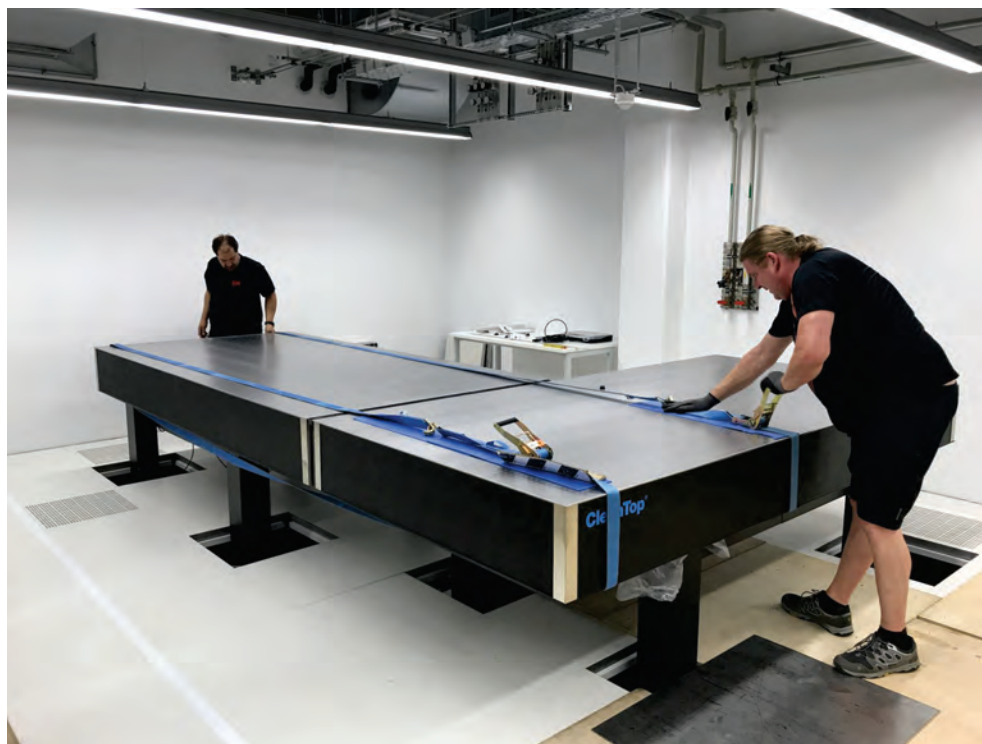
Fig. 11: Joining of optical tops; photo credit: TMC
