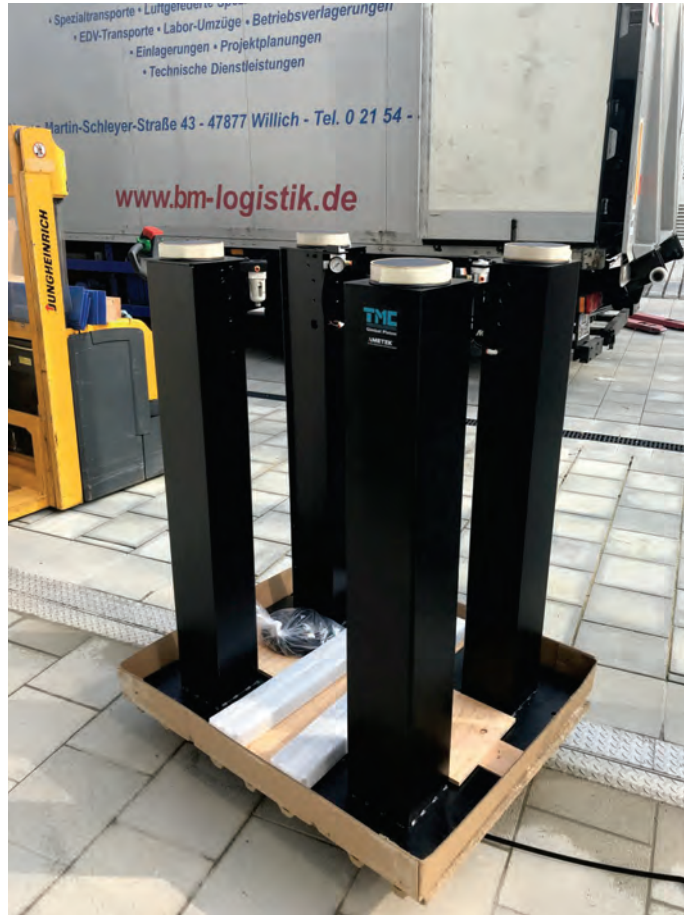
Fig. 3: Custom TMC 1200 mm high posts with Gimbal Piston Isolators, photo credit: TMC
