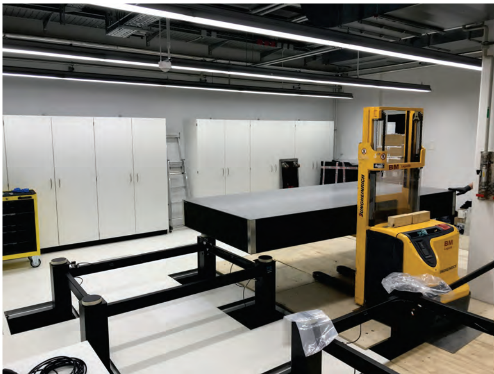
Fig. 9: Installation of first optical top; photo credit: TMC
